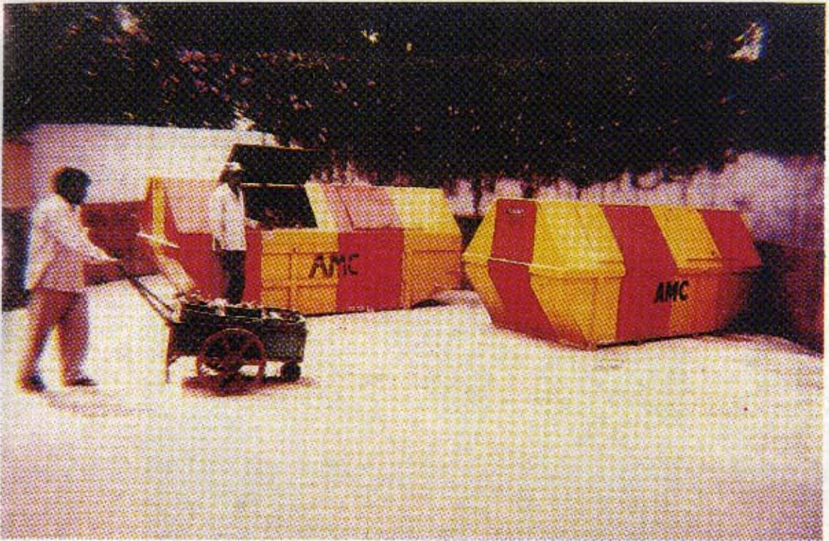
WASTE COLLECTED FROM THE DOORSTEP BEING TAKEN TO WASTE STORAGE DEPOT (CONTAINER)
