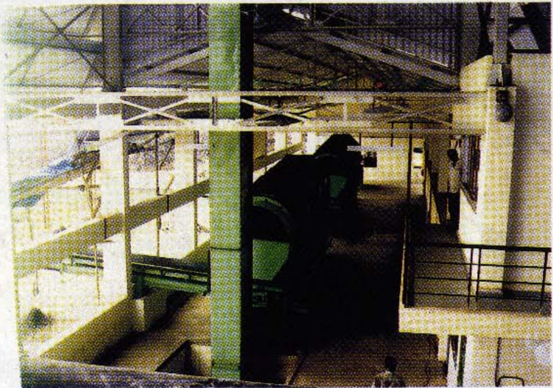
SIEVING OF COMPOSTED MATTER AT THE COMPOST PLANT
